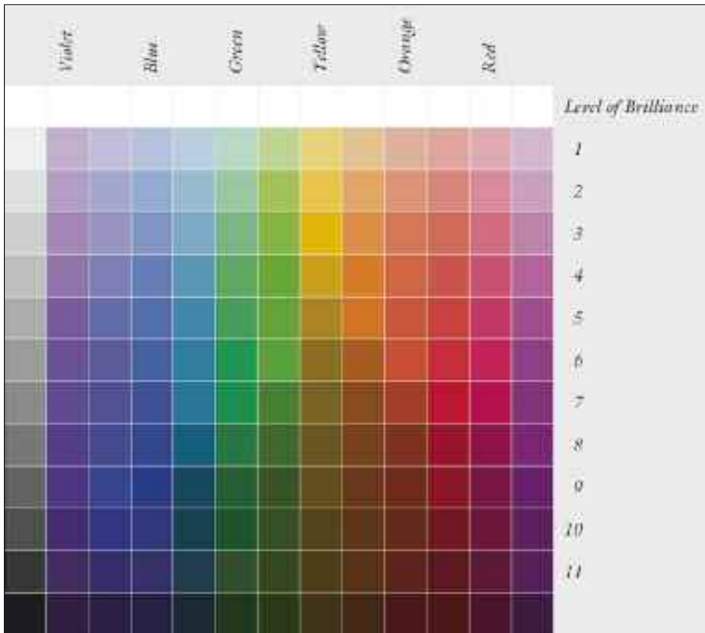
Figure 9. Colour Chart. The left hand column has white at the top, Black at the bottom and 10 evenly graduated greys in between. To its right are the 12 colours of the Colour Circle, white at the top, black at the bottom such that each horizontal line has each colour of the same level of brilliance.
